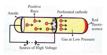
Fig 3.2: Formation of positive rays in the immersion tube.
