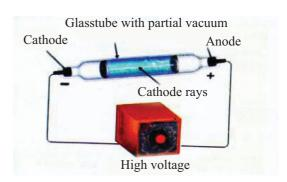
Fig. 3.1: Formation of Cathode Rays in the Immersion tube
