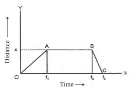
Fig. 9.6 Distance -time graph of the nonuniform velocity
