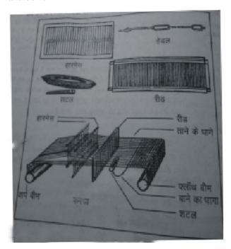
Figure: 21.1 (Different Part of Loom)
