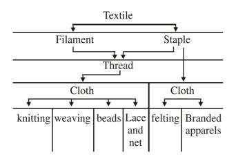
Yarn is prepared using long and short threads. Formation of threads is known as spinning.
